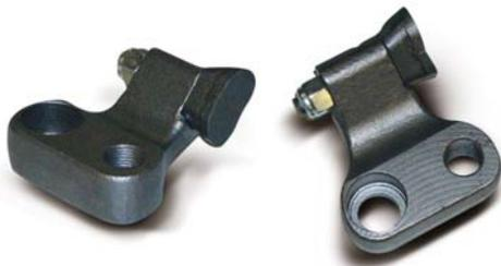
**Yellow Jacket cutter system**, a Vermeer exclusive, offers faster, easier serviceability, along with almost double the pocket and tooth life of other systems. Teeth mounted on the side of the cutter wheel in a 4.5" (11.4 cm) wide radial band allow a deeper cut on each pass through the stump.
