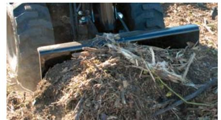
**The optional 34" (86.4 cm) wide chip blade easily moves chips around the jobsite, reducing manual cleanup time. Its rounded lower edge reduces turf damage.**
