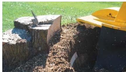
**The cutter wheel can achieve cutting heights of 31" (78.7 cm) above ground and 25" (63.5 cm) below grade. As the boom drops from the fully raised position, the wheel moves away from the machine, increasing the cutting width and boosting productivity without having to reposition the unit.**
