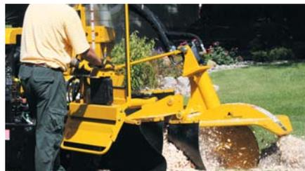
**Direct-drive hydrostatic motor** powers the cutter wheel, eliminating the need for clutch and belt-drive maintenance. The inline drive system between the motor and gearbox is connected by a driveshaft with u-joints, eliminating side loads and prolonging seal and motor-component life.
