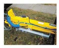
A 60" (152.4 cm) tongue extension helps reduce the amount of repositioning needed on a jobsite.
